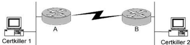
Certkiller 1 and Certkiller 2 are on Ethernet LANs in different buildings. A serial line is installed between two Cisco routers using Cisco HDLC serial line encapsulation. Routers A and B are configured to route IP traffic. Certkiller 1 sends a packet to Certkiller 2. What is the destination MAC address of the packet on Certkiller 's 1 Ethernet?
